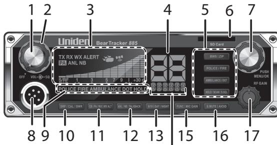
1. **Volume Control** knob with **Power On/Off**. Turn the knob clockwise until it clicks to turn power on. Continue turning the knob clockwise to increase the volume. Turn the **Volume Control** knob counterclockwise to decrease the volume or until it clicks to turn power off.
